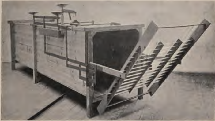
Fig. 23.—Apparatus for testing aeroplanes, condensers, etc., in an air blast. The opening is 3 feet square. Thin brass sustainers are shown in position for testing.
